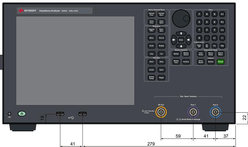
Figure 7. Main unit dimensions (front view, in millimeters).
