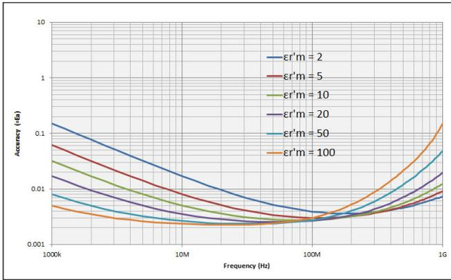
Figure 16. Dielectric loss tangent ( $\tan\delta$ ) accuracy vs. frequency (at  $t = 0.3$  mm, typical)<sup>1</sup>
