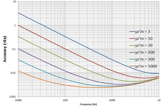
Figure 48. Permeability loss tangent ( $\tan\delta$ ) accuracy vs. frequency (at  $F = 0.5$  mm, typical) <sup>1</sup>
