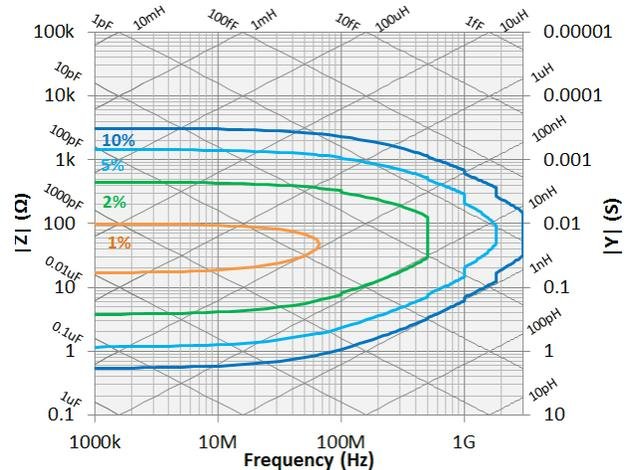
Figure 4.  $|Z|$ ,  $|Y|$  Measurement accuracy when open/short/load calibration is performed. Oscillator level =  $-33$  dBm. Point averaging factor  $\leq 7$  within  $\pm 5$  °C from the calibration temperature.
