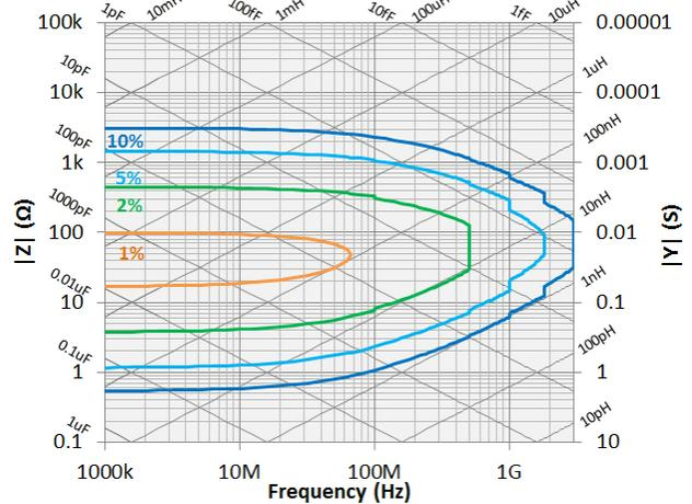
Figure 34.  $|Z|$ ,  $|Y|$  measurement accuracy when open/short/load calibration is performed. Oscillator level =  $-33 \text{ dBm}$ . Point averaging factor  $\leq 7$  within  $\pm 5^\circ\text{C}$  of calibration temperature.
