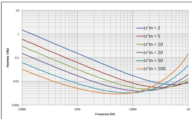
Figure 18. Dielectric loss tangent ( $\tan\delta$ ) accuracy vs. frequency (at  $t = 3$  mm, typical)<sup>1</sup>
