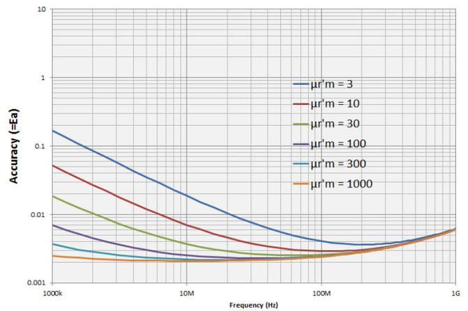
Figure 50. Permeability loss tangent ( $\tan\delta$ ) accuracy vs. Frequency (at  $F = 10$  mm, typical) <sup>1</sup>
