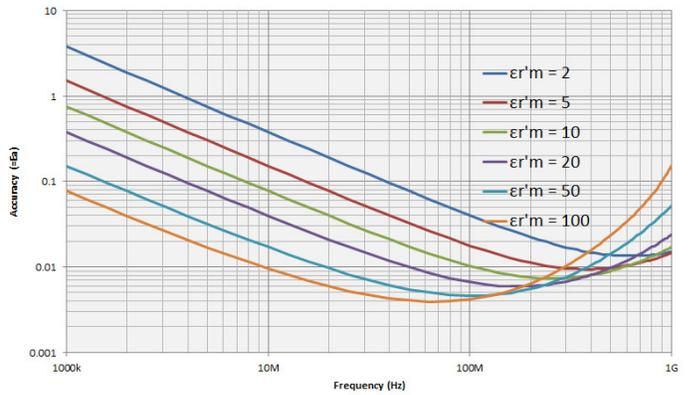
Figure 41. Dielectric loss tangent ( $\tan\delta$ ) accuracy vs. frequency (at  $t = 3$  mm, typical) <sup>1</sup>
