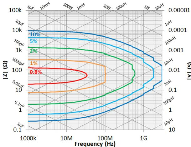
Figure 3.  $|Z|$ ,  $|Y|$  Measurement accuracy when open/short/load calibration is performed. Oscillator level =  $-33$  dBm. Point averaging factor  $\geq 8$  within  $\pm 5$  °C from the calibration temperature.
