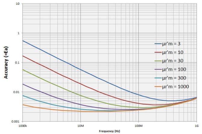
Figure 49. Permeability loss tangent ( $\tan\delta$ ) accuracy vs. frequency (at  $F = 3$  mm, typical) <sup>1</sup>
