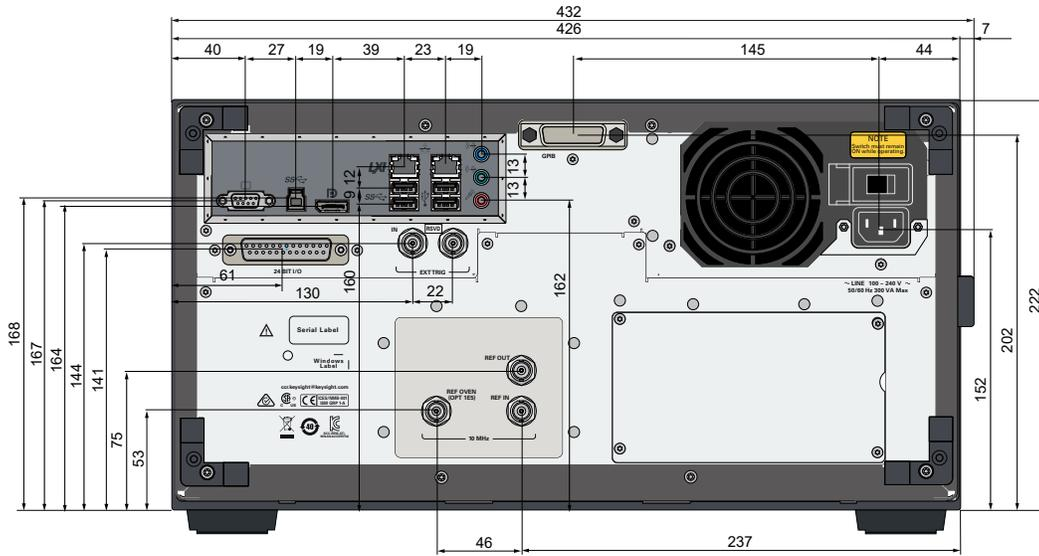
Figure 8. Main unit dimensions (rear view, in millimeters).
