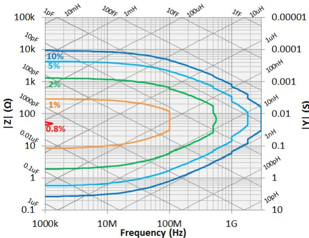
Figure 32.  $|Z|$ ,  $|Y|$  measurement accuracy when open/short/load calibration is performed. Oscillator level  $-13 \text{ dBm}$ ,  $-3 \text{ dBm}$ . Point averaging factor  $\leq 7$  within  $\pm 5^\circ\text{C}$  of calibration temperature.
