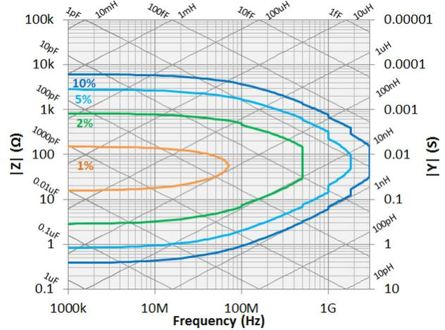
Figure 33.  $|Z|$ ,  $|Y|$  measurement accuracy when open/short/load calibration is performed. Oscillator level =  $-33 \text{ dBm}$ . Point averaging factor  $\geq 8$  within  $\pm 5^\circ\text{C}$  of calibration temperature.
