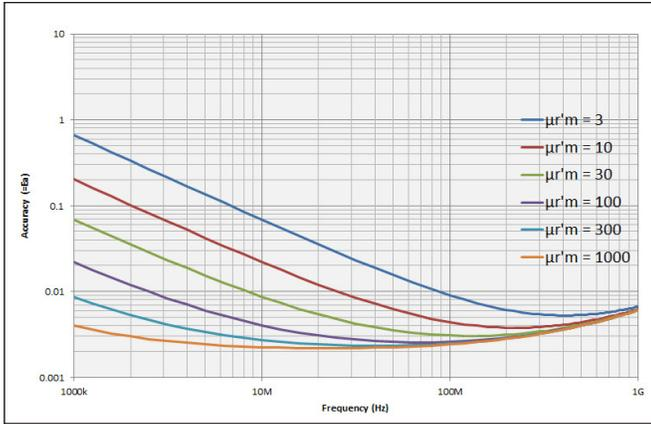
Figure 25. Permeability loss tangent ( $\tan\delta$ ) accuracy vs. frequency (at  $F = 0.5$  mm, typical) <sup>1</sup>
