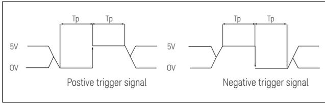
Figure 6. Definition of pulse width ( $T_p$ ).
