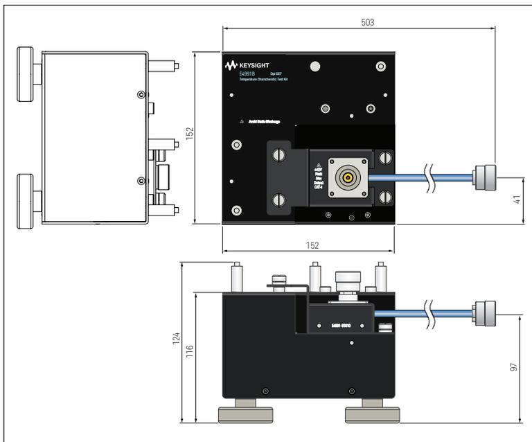
Figure 11. Option E4991B-007 test head dimensions (in millimeters).
