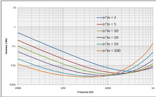
Figure 17. Dielectric loss tangent ( $\tan\delta$ ) accuracy vs. frequency (at  $t = 1$  mm, typical)<sup>1</sup>
