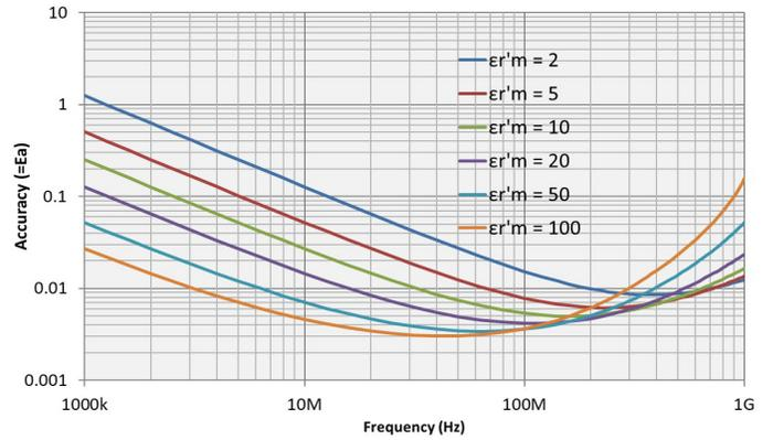
Figure 40. Dielectric loss tangent ( $\tan\delta$ ) accuracy vs. frequency (at  $t = 1$  mm, typical) <sup>1</sup>
