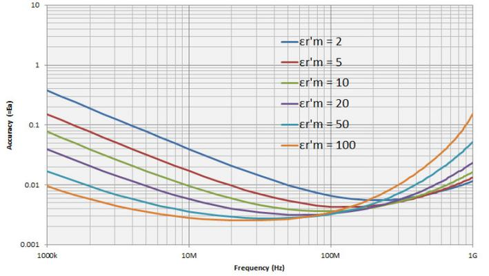
Figure 39. Dielectric loss tangent ( $\tan\delta$ ) accuracy vs. frequency (at  $t = 0.3$  mm, typical) <sup>1</sup>
