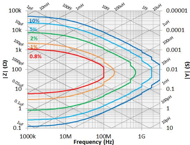
Figure 1.  $|Z|$ ,  $|Y|$  Measurement accuracy when open/short/load calibration is performed. Oscillator level =  $-13 \text{ dBm}$ ,  $-3 \text{ dBm}$ . Point averaging factor  $\geq 8$  within  $\pm 5 \text{ }^\circ\text{C}$  from the calibration temperature.
