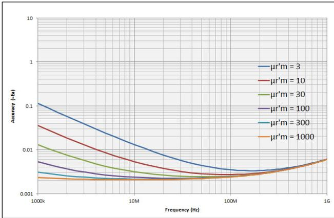
Figure 26. Permeability loss tangent ( $\tan\delta$ ) accuracy vs. frequency (at  $F = 3$  mm, typical) <sup>1</sup>
