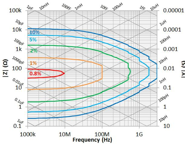
Figure 31.  $|Z|$ ,  $|Y|$  measurement accuracy when open/short/load calibration is performed. Oscillator level =  $-13 \text{ dBm}$ ,  $-3 \text{ dBm}$ . Point averaging factor  $\geq 8$  within  $\pm 5^\circ\text{C}$  of calibration temperature.
