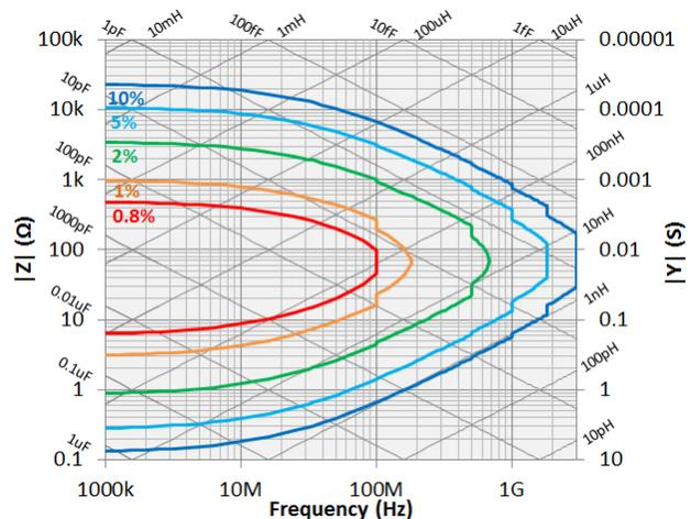
Figure 2.  $|Z|$ ,  $|Y|$  Measurement accuracy when open/short/load calibration is performed. Oscillator level  $-13 \text{ dBm}$ ,  $-3 \text{ dBm}$ . Point averaging factor  $\leq 7$  within  $\pm 5 \text{ }^\circ\text{C}$  from the calibration temperature.
