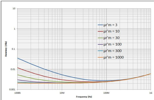
Figure 27. Permeability loss tangent ( $\tan\delta$ ) accuracy vs. frequency (at  $F = 10$  mm, typical) <sup>1</sup>
