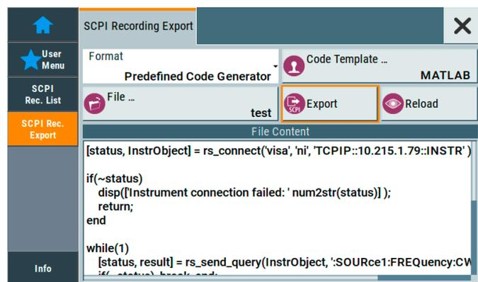
The R&S®SMBV100B helps users quickly and correctly create remote control programs. The instrument's built-in SCPI macro recorder with code generator can automatically record all manual settings and create an executable MATLAB® script. The R&S®SMBV100B therefore helps minimize the time required for test automation, saving development resources.
